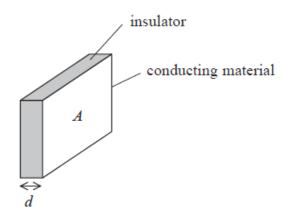
The capacitor has a capacitance  $0.1~\mu F$  and is charged to a p.d. of 100 V by connecting it to an electrical supply.
