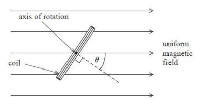
(a) The coil has 200 turns and an area of  $2.0 \times 10^{-4}$  m<sup>2</sup>.
