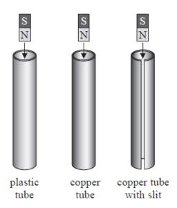
(a) The teacher releases a magnet from rest at the top of the plastic tube and it takes 0.45 s to fall through the tube.
