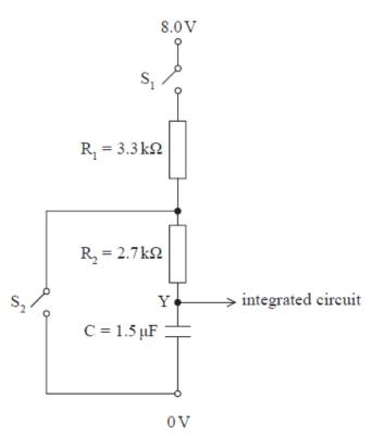
When the potential at Y is  $8.0\,V$ , the switch  $S_2$  is closed.
