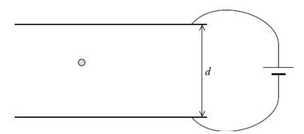
When the p.d. is 0 V the oil drop accelerates to terminal velocity. The p.d. is increased. It is observed that at a particular p.d. V the oil drop stops falling and remains stationary between the
