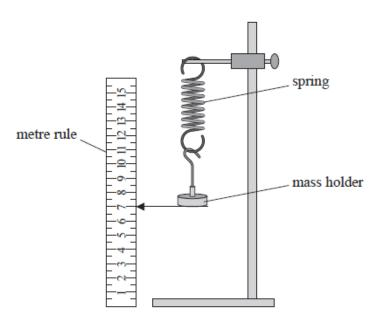
The position of the bottom of the mass holder was recorded. The spring was stretched by adding masses to the mass holder and the new positions were recorded. The extension of the spring each time was calculated.
