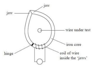
The 'jaws' of the clamp are opened, placed around the wire carrying the current and then closed. Inside the 'jaws' is an iron core with a coil of wire wrapped around it.
