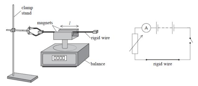
With the switch open, the balance was set to zero. When the switch was closed a current *I* in the circuit was recorded by the ammeter and the reading on the balance increased.
