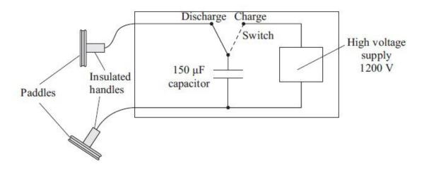
(a) The 150 µF capacitor is first connected across the 1200 V supply
