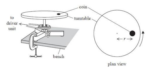
The student switched on the driver unit and increased the rate of rotation until the coin slid off the turntable. He read the angular velocity  $\omega$  of the turntable from a digital display on the driver
