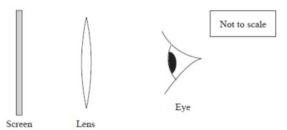
For a particular user of the headset, the image of the screen must be at least 16 cm from the eye and have a magnification of at least 3.0.
