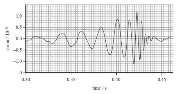
Gravitational waves alternately compress and stretch matter by very small amounts as they pass through.
