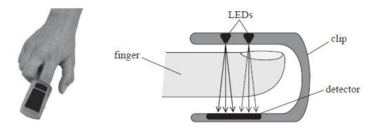
The intensity I of electromagnetic radiation received by the detector, after passing through a thickness x of blood, is given by
