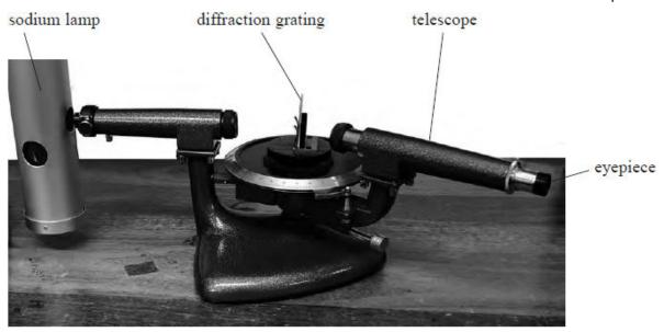
The spectrometer allows parallel rays of light to be passed through a diffraction grating and the resulting angles of diffraction to be measured.
