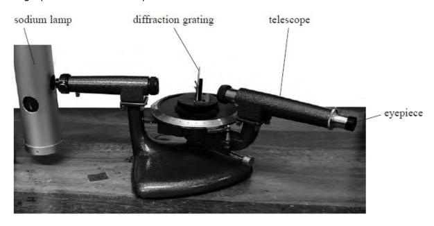
The spectrometer allows parallel rays of light to be passed through a diffraction grating and the resulting angles of diffraction to be measured.
