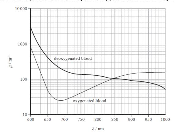
The oximeter determines  $I/I_0$  the fraction of radiation transmitted at each wavelength.
