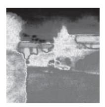
The photograph shows the result when someone tries to take an infrared photograph of the same scene through a window. The image does not show the outdoor scene but does show an image of the photographer.
