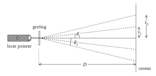
The diagram shows the first two diffracted orders where  $x_1$  and  $x_2$  are the distances of the maxima for these orders from the central maximum of the diffraction pattern.
