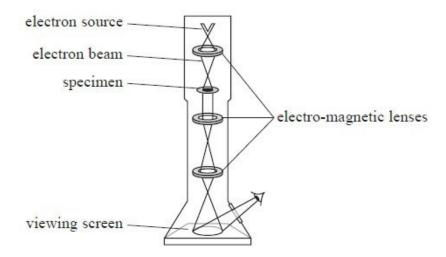
Due to the wave nature of electrons, diffraction occurs which can blur the image. To reduce this effect when viewing a smaller object the beam must contain
