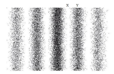
The path difference for electrons arriving at band X from the separate slits was  $2.5 \times 10^{-1}$  m. For electrons arriving at band Y the path difference was  $5.0 \times 10^{-1}$  m.
