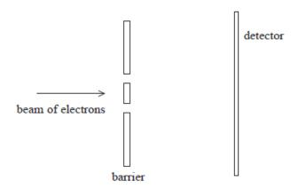
A beam of electrons was directed at a barrier with two slits.
