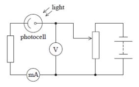
The student illuminates the photocell with light of known frequency f. A current is produced in the circuit due to the emitted electrons. He adjusts the potential difference, using a potential divider, until the reading on the milliammeter is zero and records the corresponding reading  $V_s$  on the voltmeter. He repeats this procedure for other frequencies of light.
