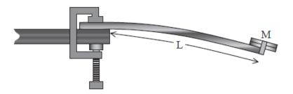
When M is displaced, the period of oscillation T of the cantilever is related to L and the Young modulus E of the material of the metre rule by the following equation:
