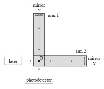
The laser beam is split into two at B, one beam travelling to one mirror and the other beam travelling to the other mirror. After reflection at the mirrors, the beams are recombined at B and reach the photodetector. The photodetector measures the intensity of the incident light.
