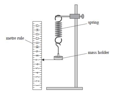
The position of the bottom of the mass holder was recorded. The spring was stretched by adding masses to the mass holder and the new positions were recorded. The extension of the spring each time was calculated.
