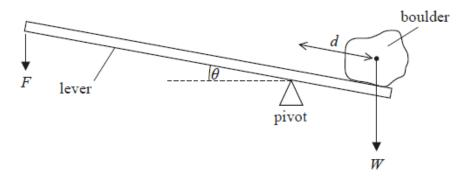
The centre of gravity of the boulder is a distance d from the pivot. The angle of the lever to the horizontal is  $\theta$ .
