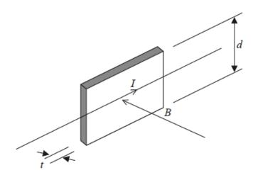
Electrons collect at the top edge of the slice and the bottom edge becomes positively charged. As a result a potential difference known as a Hall voltage  $V_{\rm HALL}$  develops.
