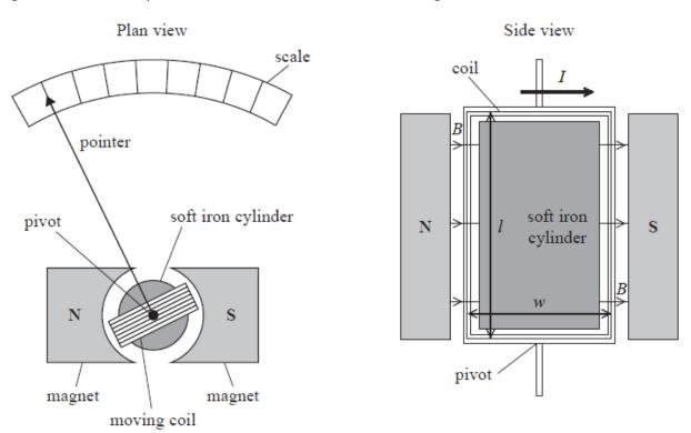
The fixed soft iron cylinder and magnets produce a uniform magnetic field of magnetic flux density B. The coil is able to rotate within this magnetic field. The coil has width w and length I. There is a current I in the coil in the direction shown in the side view diagram.
