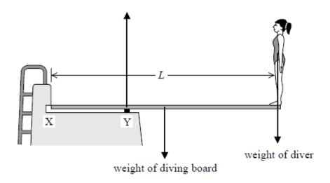
The diving board has a length L of 3.6 m and is fixed at the end labelled X. It is supported at position Y which is 0.9 m from X. The diving board is uniform and has a weight of 390 N.
