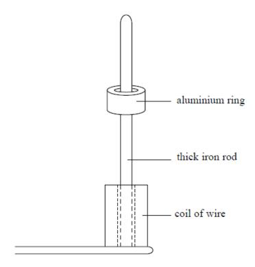
The current is switched off and the aluminium ring comes to rest on top of the coil. The supply to the coil is changed and a direct current (dc) is switched on. An upwards force F acts on the ring for 0.05 s accelerating it to a final speed, v. The ring then moves freely through a height of 30 cm.
