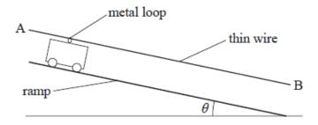
The student uses a protractor to measure the angle  $\theta$  between the ramp and the horizontal and records a value of  $4^{\circ}$  with an uncertainty of  $\pm 1^{\circ}$ .
