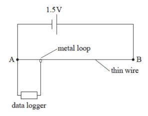
Explain how the potential difference recorded by the data logger will vary as the loop moves along the length of the wire AB.
