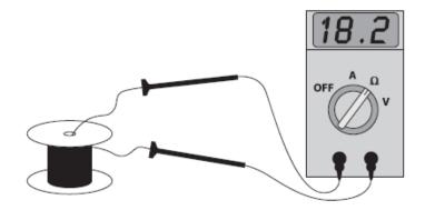
The diameter of the wire was measured as 0.27 mm  $\pm$  0.01 mm. The length of the wire was measured as 1.25 m  $\pm$  0.05 m.
