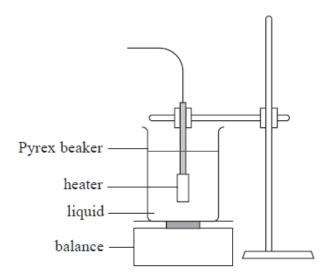
The student monitored the mass of the beaker and the liquid m over the time t for which the liquid was boiling. Her results are plotted on the graph.
