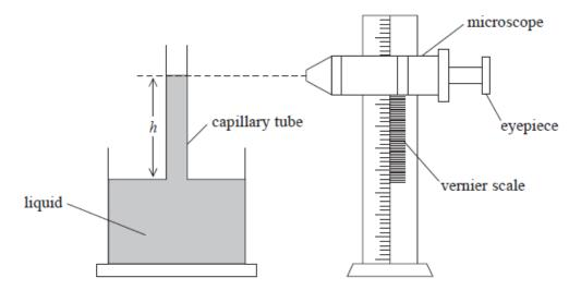
The student used a capillary tube with an internal radius r equal to 0.10 mm and recorded the following readings from the vernier scale.
