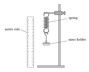
In another experiment, the student displaced the mass vertically each time a mass was added to
