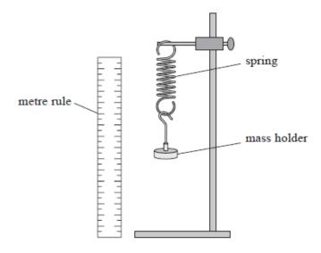
In another experiment, the student displaced the mass vertically each time a mass was added to the spring. He used a stopwatch to determine the period of vertical oscillations of each mass.
