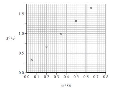
When determining the period of oscillation for each mass, the student measured the time for 20 oscillations. He repeated this measurement to obtain a mean time for 20 oscillations.
