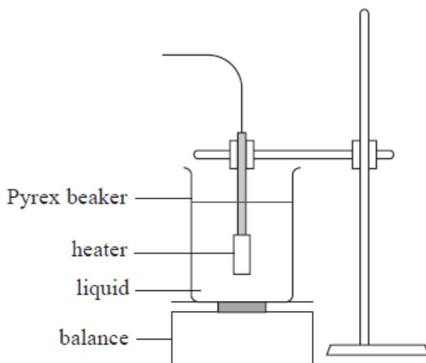
She connected the heater into a circuit and took measurements of the potential difference  $V$  and the current  $I$  for the heater.
