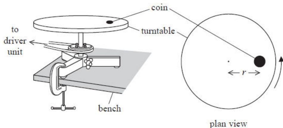
The student switched on the driver unit and increased the rate of rotation until the coin slid off the turntable. He read the angular velocity  $\omega$  of the turntable from a digital display on the driver unit. He then replaced the coin in the original position on the turntable and repeated the
