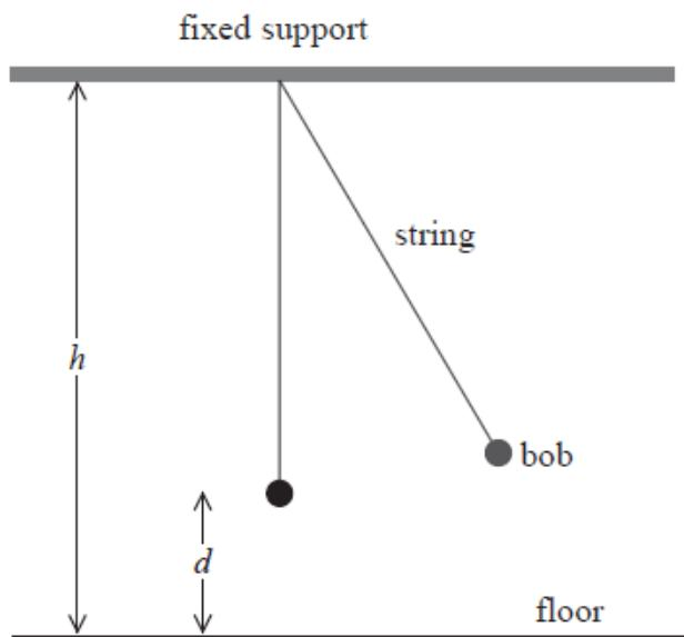
As the student was unable to measure the length of the pendulum directly, she measured the distance  $d$  from the bob to the floor.
