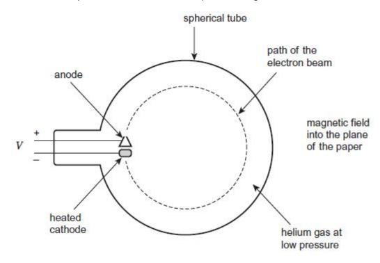
Electrons are accelerated by a potential difference (pd) V applied between the cathode and anode. A magnetic field of known flux density B, directed into the plane of the diagram, causes the electrons to move in a circular path.
