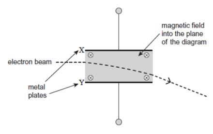
(a) The diagram shows the path of the electron beam when the magnetic field is applied and the pd between X and Y is zero.
