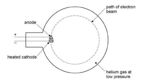
Electrons are emitted by the cathode by thermionic emission. They are accelerated by the potential difference between the cathode and anode. The tube contains helium gas at a low pressure and the gas emits light to show the path of the electron beam.
