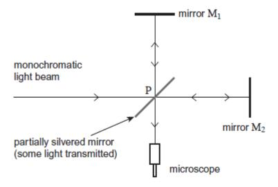
In the apparatus, light waves reflected by the mirrors  $M_1$  and  $M_2$ , meet at P so that they superpose and produce interference fringes. These are observed using the microscope.
