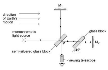
It was predicted that when the interferometer was rotated through 90° the fringe pattern would shift by 0.4 of the fringe spacing.
